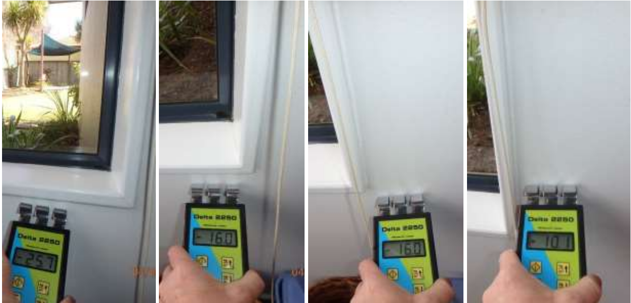
Moisture readings are not high but should be monitored for mould or mildew growth.
