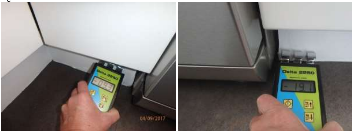
Each side of the dishwasher with a raised reading on the right
